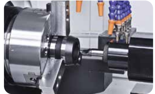
Single Grinding Spindle and Turning Tool Structure
